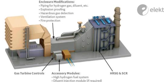
CCGT plant does not require any modernisation, if H<sub>2</sub> share in CH<sub>4</sub>-H<sub>2</sub> mixture does not exceed 5% (volume).
